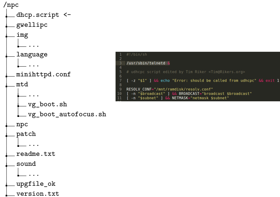
Fig. 9. Content of the file system left. On the right, the added line to create the telnet back door.
